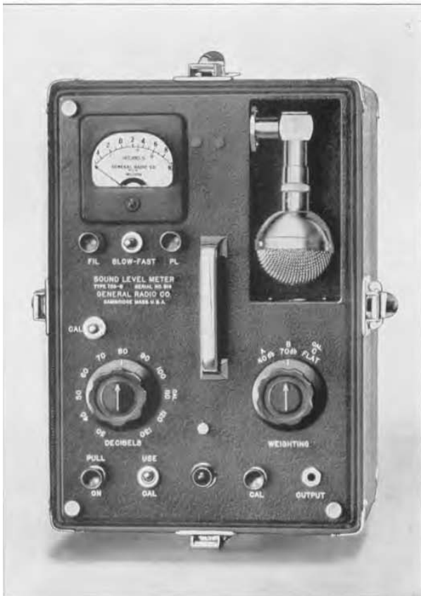
FIGURE 7. Panel View of the General Radio TYPE 759-B Sound-Level Meter.
